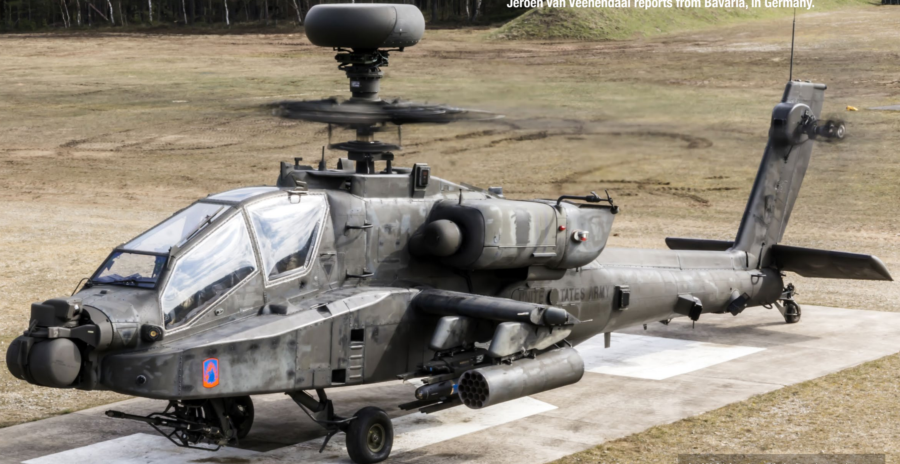
An AH-64 Apache, with the Longbow radar, sits with the rotors spinning, preparing to take off. Photo by Roelof-Jan Gort
